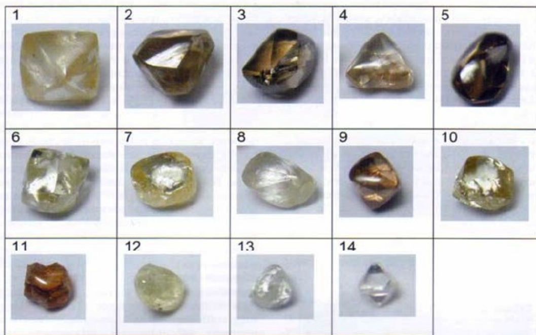
Fig. 1. Fourteen specimens of rough diamond (KTM 1-14) acquired from Banjarmasin-Martapura that weighed from 0.03 to 1.82 ct and range in colour from colourless to light yellow, yellow and brown. Note: KTM 11 was subsequently shown to be a zircon.
